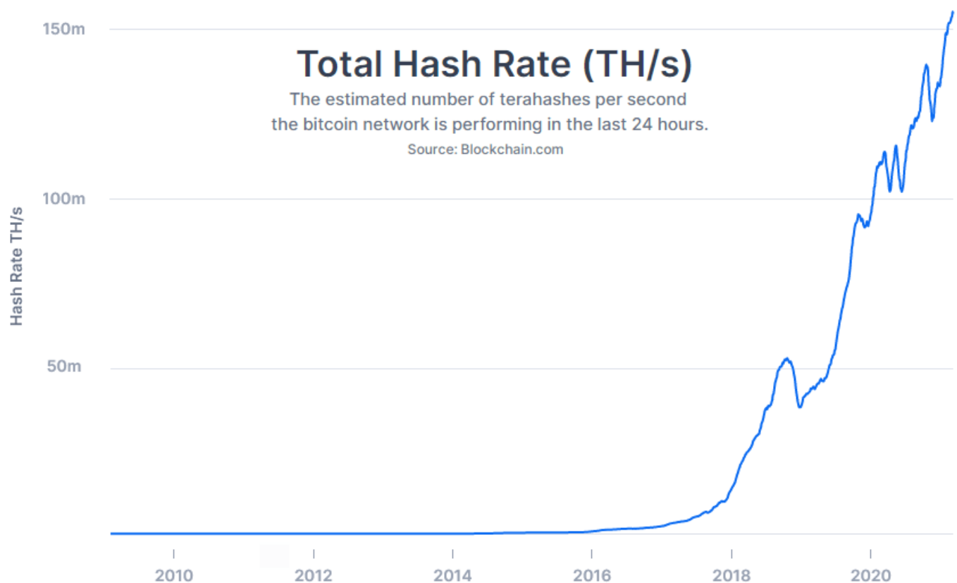
Figure 69. Total hashing power, terahashes per second (TH/sec) (chart on a linear scale)
