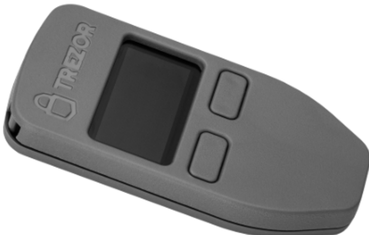
Figure 26. A Trezor device: a bitcoin HD wallet in hardware
